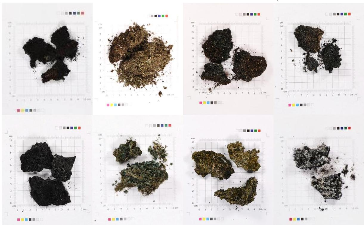
Figure 2: Selected slag samples from practical combustion tests (f.l.t.r: upper row: stem wood spruce, hardwood mixture, short rotation willow/spruce (#1), short rotation willow/spruce (#2), lower row: miscanthus, vineyard prunings, corn cobs, DDGS)
