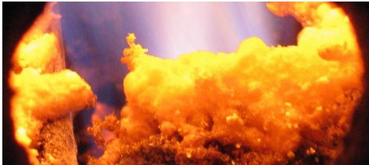
Figure 3: View on slag formation during combustion of corn cobs fuel in a small scale combustion appliance
